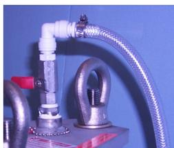
Air purge valve and drain tubing
