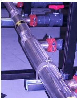
Stainless Steel Paint TruFlow Paint Manifold, note tapered diameters
