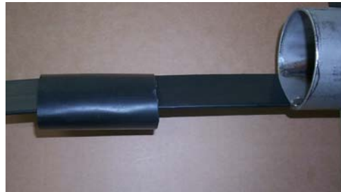
Picture #4 Shows the loose piece of shrink tubing evenly over electrical connection.
