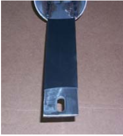
Picture #1 Electrode with shrink tubing.
