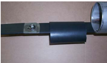
Picture #3 Shows loose piece of shrink tubing on electrode tab.
