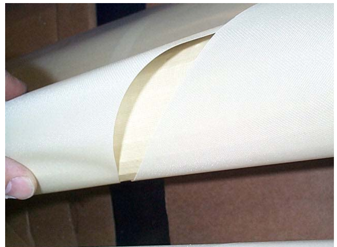
Picture 2 Loose wrap on mishandled membrane shell.
