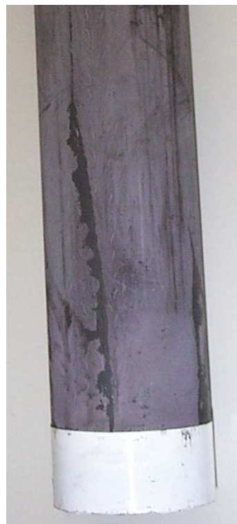
Figure 2. (Typical Loss of Coating)
