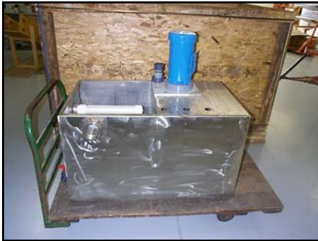
Partially assembled Cell Circulation Tank
