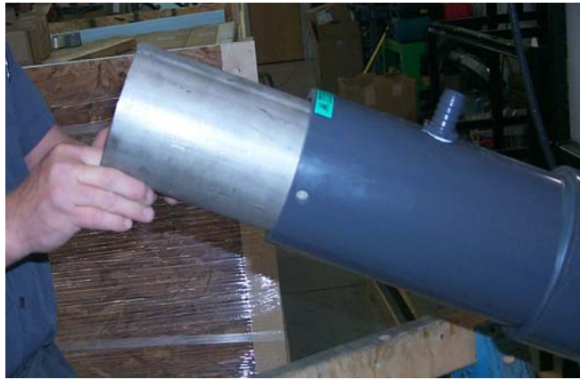
#2 Slowly insert the SS Electrode into the Membrane Shell. Do not drop the electrode into Membrane Shell as damage may occur.
