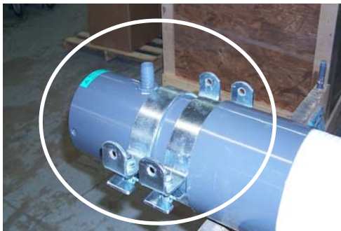
#5 Place metal brackets on neck (located at the collar end) of T5.
