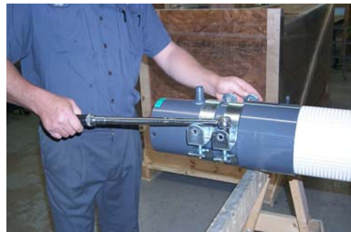
#6 Tighten metal clamps to 21 FT/LBS.
