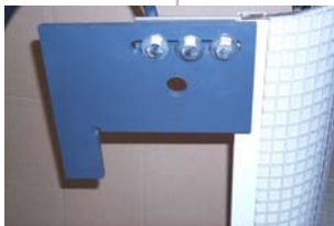
Photo #1 Showing Bracket PN 100111 installed with 3 x 1/2" Bolt hardware. Round hole is for lifting
