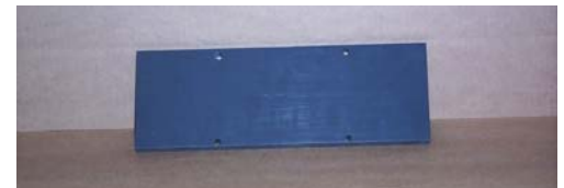
Photo #2 Shows (4) pre- drilled holes in PVC plate.
