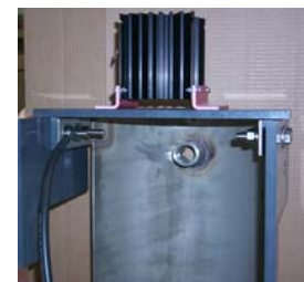
Photo #4 Shows heat sink assembly mounted to the One+ C-Cell.
