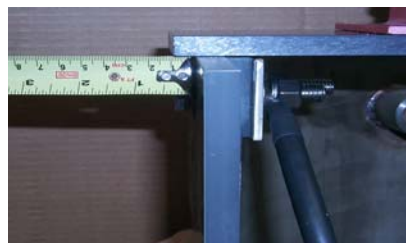
Photo #3 Shows PVC plate with 10mm overlap.
