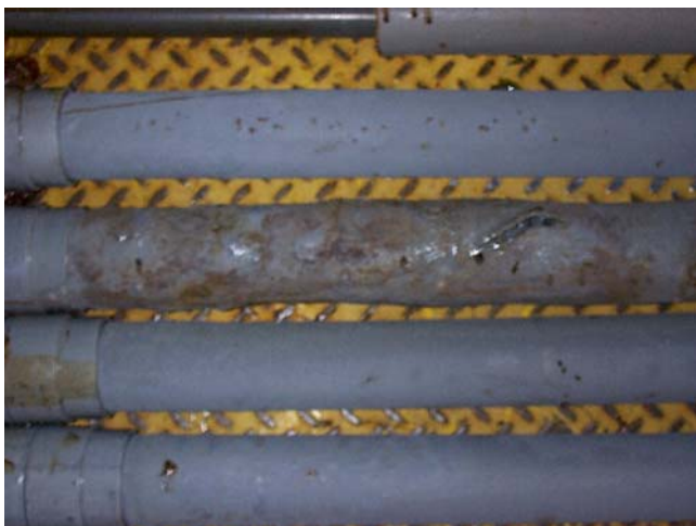
Heat Stressed ED Core Cell, middle Cell (notice the cut on this cell too)
